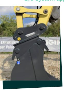
The main added value of the Evo system relates to safety and operating efficiency, responding to the latest safety prerequisites introduced by the EN474 standard. With this innovative system, the operator can check whether the quick coupler has engaged correctly without leaving their seat in the cab. This is achieved by means of a dual indicator system which informs the operator whether the quick coupler is fully connected to the adapter.
