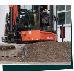
The excavator blade control (EBC) is an automated control system for the excavator blade. Grading jobs can be done with the blade instead of the bucket, when the EBC in installed giving the possibility to do levelling jobs supported by an automated control system.
