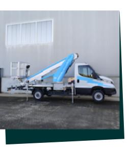
Mounted on an Iveco eDaily 35S10 Full Electric truck of 3.5 t GVW, a telescopic platform providing a working height of 16.2m and a load capacity of 80kg at its maximum horizontal outreach of 11.2m, rising to 250kg at 7.4m outreach. At a length of 7,123mm and height of 2,740mm when closed, it has straight line stabilizers with front and rear vertical descent, making it a vehicle easy to position even in tight spots.
