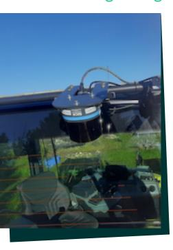
BOMAG Emergency Brake Assist is a technology designed for road construction machines that prevents collisions while protecting the hot asphalt surface from damage. The machine continuously scans its surroundings for perfect coverage. System is able to detect potential hazards before they occur. This allows for the early application of automatic deceleration strategies.
