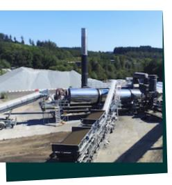
The TSX is a new continuous asphalt plant, ecological, unique in the world, capable of recycling from 0 to 70% of recycled asphalt pavement (RAP) coming from road maintenance with just one drum, while ensuring environment respect and high-quality HMA.
