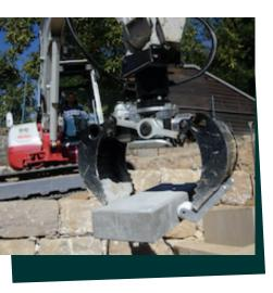
The DMS sorting grab SG is the first grab on the market with a fully enclosed plunger cylinder for digging and grabbing with excavators and loading cranes. The distinctiveness lies in the development of the patented, double-acting hydraulic cylinder. The reduced tare weight made possible by the unique, compact design allows any hydraulic excavator to carry more payload.
