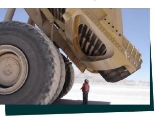
**Duratray's Smart Tray (ST) is the most advanced dump tray for mining and construction trucks.** The ST can monitor its condition (structural and wear) automatically and report to the user online and in real time.
